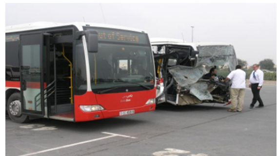
An exemplar vehicle used for comparison purposes in a bus crash investigation
