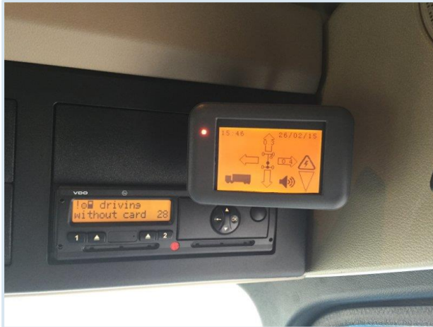
Figure 11 - Example of Inclinometer (TSafe Tipper Safety System)
