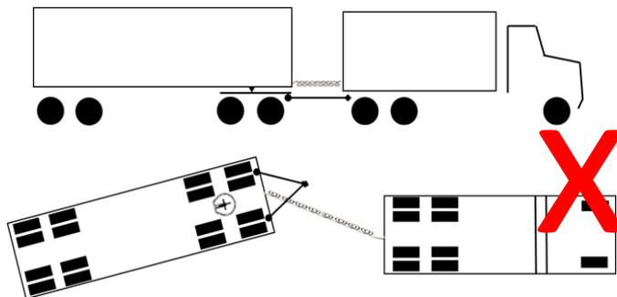
Potential Suzi coil stretch after trailer decoupling.
