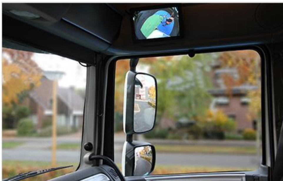
Figure 7-3: Example of Orlaco Cornereye® installation
