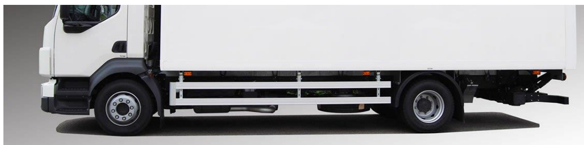
Figure 10-1: Example of HGV side guard. Source: (Nationwide Trailer Parts, 2018)
