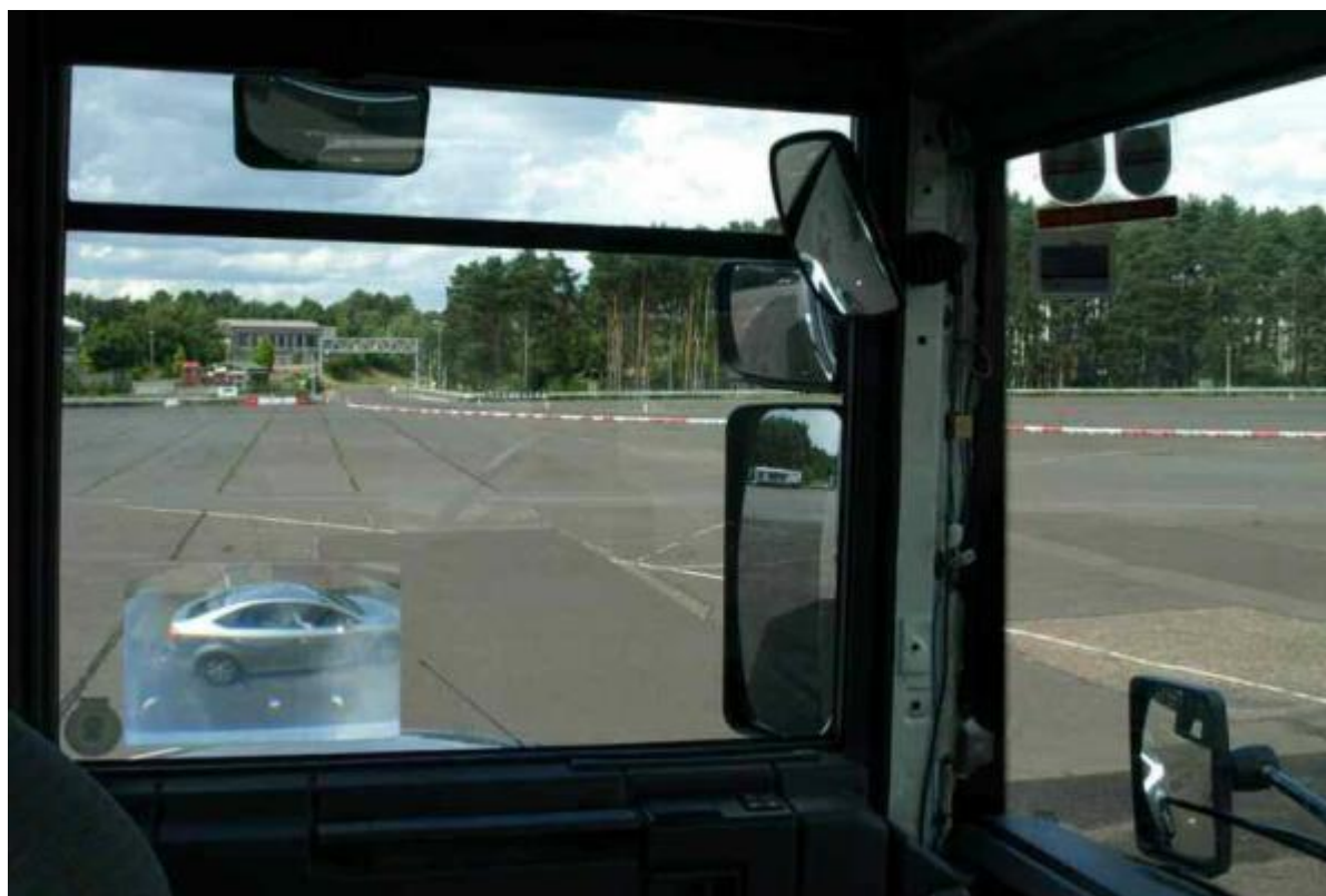
Figure 5-2: Image of a test vehicle equipped with two additional blind spot mirrors and a Fresnel lens
