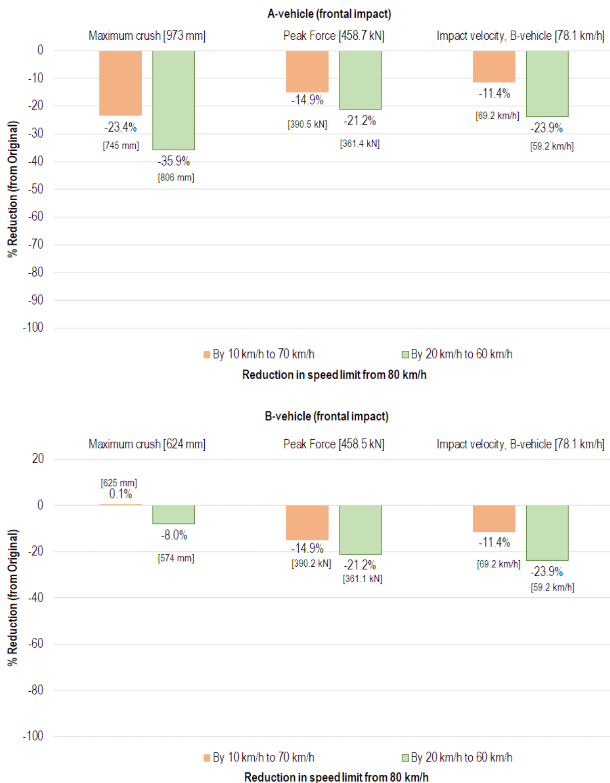
FIGURE E.3 CHANGE IN MAXIMUM CRUSH, PEAK FORCE, AND IMPACT VELOCITY BY SPEED LIMIT CHANGES FOR THE A-VEHICLE AND THE B-VEHICLE RELATIVE TO THE ACTUAL CRASH SCENARIO
